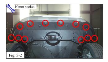
(b) From under the vehicle, remove the (12) screws (Fig. 3-2).
