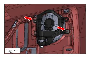
(b) Using #2 Phillips screwdriver, remove the (1) inner and (1) outer mounting screws and save for re-use (Fig. 5-2).
