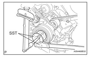
(c) Using SST, install the damper bolt.
