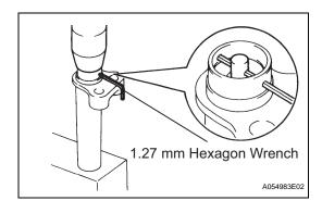
(2) Using the crankshaft damper bolt, turn the crankshaft to align the timing marks of the crankshaft timing pulley and oil pump body.
