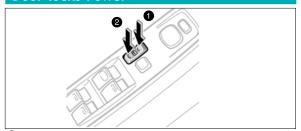
To lock Push down on the front of the switch.To unlock Push down on the back of the switch.
