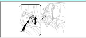
To lock the inside handle Move the lever to "LOCK," allowing the door to be opened only from the outside.
